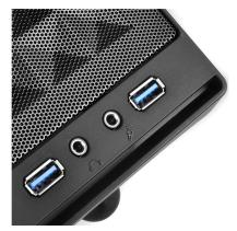
I/O ports include microphone, audio, and two USB 3.0 ports
