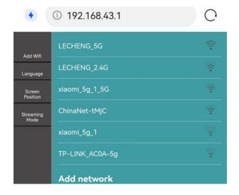
Select the network and connect in the management platform, the Receiver Unit will link to the network and show the network SSID on the middle of the screen (to get a better performance, we recommend connecting with 5G router)
