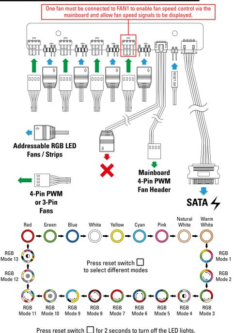
When the LED lights are off, press reset switch  $\square$  to turn on the LED lights.
