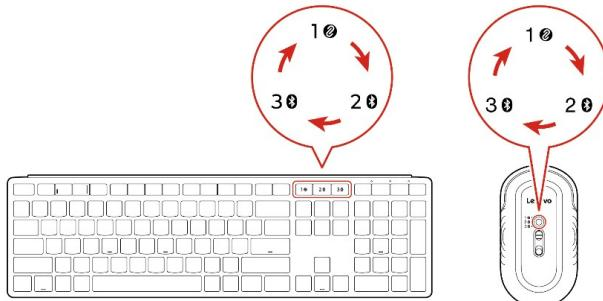
To switch between the paired devices, short-press the wireless channels connection keys or button until the desired connection indicator turns on.
