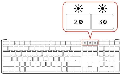
1. Press and hold the wireless channels connection key (Bluetooth channel) for two seconds (the indicator blinks quickly).
