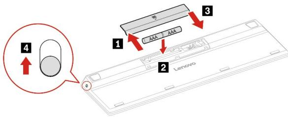
1. Remove the battery and receiver compartment cover.
