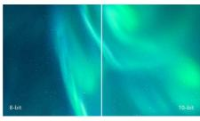
The 10-bit display delivers rich colour depth with 1.074 billion colours and 12-bit internal processing for recreating smooth, natural colours without gradations and colour banding.
