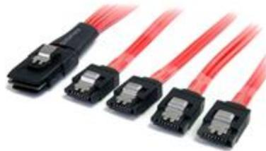
The SAS8087S450 SFF-8087 to 4x SATA SAS cable features one 36-pin plug (SFF-8087), which fans out to four SATA 7-pin receptacles, providing a reliable solution for connecting up to four SATA HDDs to a SAS controller or backplane.
