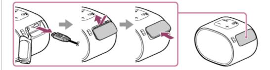
The charge indicator lights up in orange while charging. Charging is completed in about 3 hours<sup>\*</sup> and the indicator turns off.
