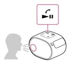
If no ring tone is heard via the speaker, the speaker may not be connected with a BLUETOOTH mobile phone with HFP or HSP. Check the connection status on the BLUETOOTH mobile phone.
