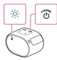
When you turn on the speaker for the first time after purchase, the power/BLUETOOTH indicator will begin to flash quickly, and the speaker enters pairing mode automatically by just pressing the () (power)/ — PAIRING
