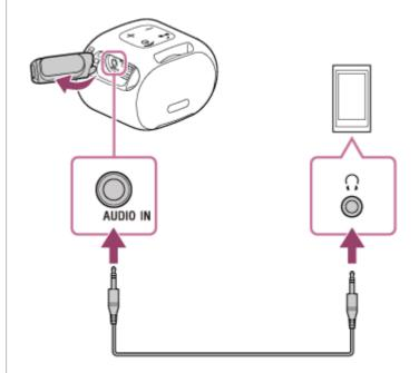
\* If you use an audio cable (with stereo mini plugs) with significant resistance, the sound may be lower. Therefore, make sure you use a cable (with stereo mini plugs) without resistance.
