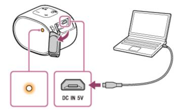
When charging is complete, close the cap securely as shown below. Placing the top side of the cap in first will allow it to close easily.
