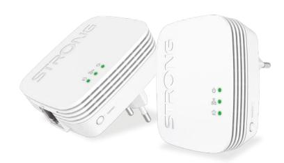
The Powerline 1000 Kit Mini which includes 2 Powerline 1000 mini adapters creates in an extremely simple way a high-speed home network using your home's existing electrical wiring at speeds up to 1000 Mbit/s.
