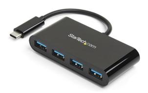
Here's a must-have accessory if you have a USB-C equipped computer but need more USB-A ports. This portable USB 3.0 hub expands your laptop or desktop connectivity by adding four USB Type-A ports through a single USB Type-C or Thunderbolt 3 port. And, because it's USB bus-powered, you don't need to connect an external power adapter, which makes travel more convenient and workstations less cluttered.
