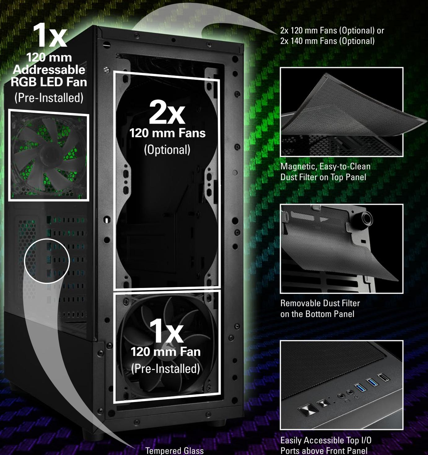
In order to keep the SK3 RGB nice and cool during operation, enough fans can be installed in the case for an optimal airflow. A 120 mm fan is already pre-installed behind the front panel, which, together with the 120 mm RGB LED fan at the rear, ensures a good circulation of air.
