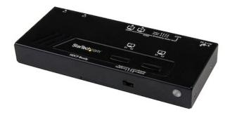
Save time and hassle by automatically switching between your HDMI audio/video sources, using the VS222HDQ 2X2 HDMI Matrix Switcher. This easy-to-use HDMI Matrix switch ensures seamless transition while switching video and display sources, with EDID copy maintaining your video resolution.
