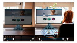
PowerSensor is a built-in 'people sensor' that transmits and receives harmless infrared signals to determine if a user is present and automatically reduces monitor brightness when the user steps away from the desk, cutting energy costs by up to 65 percent and prolonging monitor life
