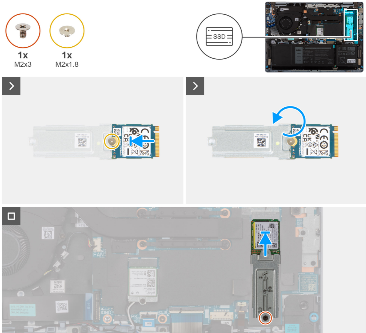
Figure 20. Installing the M.2 2230 solid state drive
