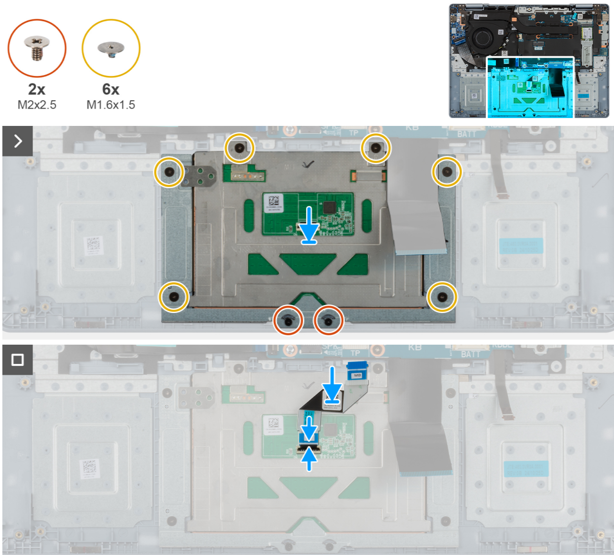
Figure 53. Installing the touchpad
