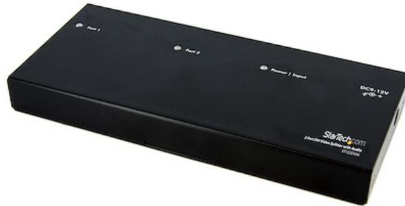
The ST122DVIA DVI splitter lets you share one DVI video and audio source on two displays and acts as a signal amplifier that allows you to locate your DVI monitors up to 33ft (10 m) away from your computer or DVI signal source.
