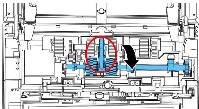
4. Close the ADF roller cover. A snap-in sound could be heard if correctly installed.
