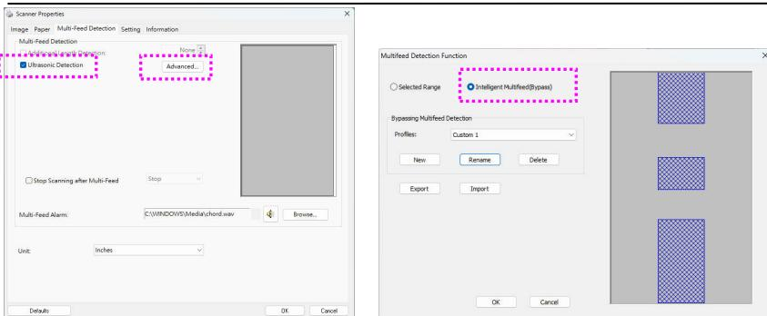
2. Click [New]. An [**Insert your paper**] dialog box will be prompted. Insert your paper with attachment on the paper to the scanner and click [**Yes**]. The scanner begins feeding the paper and the area for the attachment will be memorized by the scanner.
