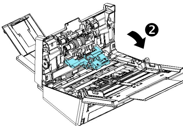
5. Press and wipe the rollers one by one. Rotate the roller until the surfaces are completely cleaned.
