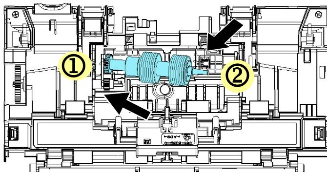
4. Insert the right end of the reverse roller to its slot.
