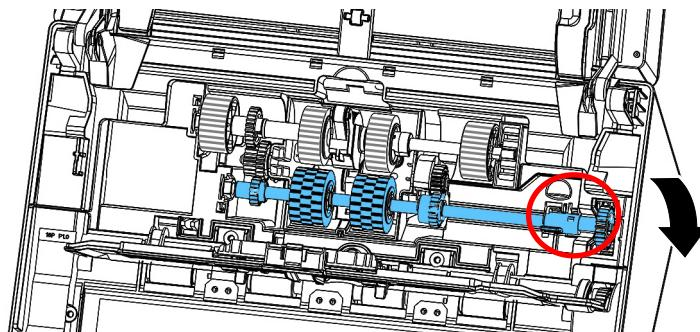
5. Detach the right end of the ADF roller from the scanner and remove the ADF roller.
