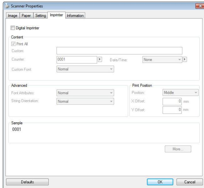
**Choice: External Imprinter, Digital Imprinter.** If you have installed an external imprinter, choose external imprinter. If you do not have an imprinter, choose digital imprinter. Note External Imprinter provides a vertical and rear-side print capability while digital printer provides a horizontal and front-side print capability.
