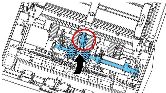
4. Move the tab of the ADF roller **DOWN** as indicated.
