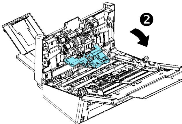
4. Press the right end of the reverse roller externally to detach it from the slot and then detach the left end from its hole.
