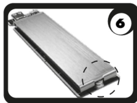
6. Put the heat sink plate on the thermal pad and align the notch to the fixture.
