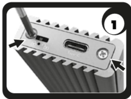
1. Remove the two screws A from the front cover.
