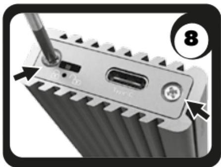
8. Reattach the front cover with the two screws A. When mounting the cover, make sure that the write protection switch is placed in the rectangular recess.
