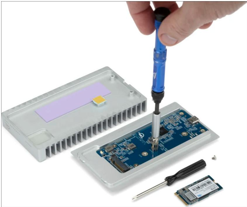
2. Carefully align the drive at a slight angle into the board connection and slide it forwards until fully seated. Once the drive is fully seated use the included drive screw to secure the drive.
