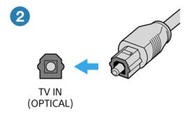
When there is no HDMI IN jack labeled "ARC" on your TV, use the optical digital cable (supplied) to connect an optical out jack on your TV and the TV IN (OPTICAL) jack on the Bar Speaker.
