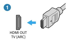
Use an HDMI cable (not supplied) to connect an HDMI IN jack on your TV and the HDMI OUT (TV (ARC)) jack on the Bar Speaker.
