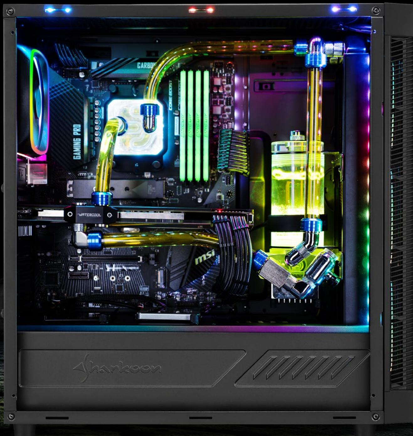
The hardware is viewable through the tempered glass front and side panels, while the power supply, HDDs and cabling disappear within the power supply tunnel or behind the mainboard tray. For a more elegant appearance and enhanced protection of the glass, the side panel has been designed without any visible screws or bolts. Instead, it is attached via thumbscrews on the rear panel of the case.
