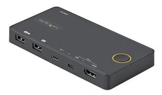
This 2-port USB-C / USB-A KVM enables you to easily switch between a USB Type-C or Thunderbolt 3 desktop/laptop computer and a USB-A and HDMI desktop/laptop computer, using a single keyboard, HDMI monitor and mouse.
