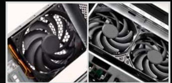
Includes three 120mm fans with filtered intake vents
