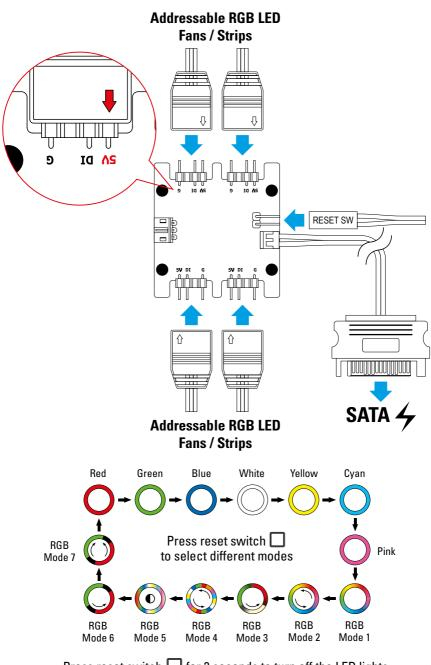
Press reset switch  $\Box$  for 2 seconds to turn off the LED lights. When the LED lights are off, press reset switch  $\Box$  to turn on the LED lights.
